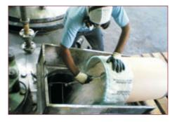
When handling drums containing nitrocellulose, do not allow them to fall or bump into each other. If possible, use a fork-lift for loading or unloading drums. To prevent sparking, do not roll or drag drums on concrete, steel floors or hard surfaces.
