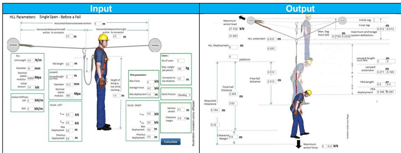
Figure 1: Sample illustration of FPSWizard for HLLS
